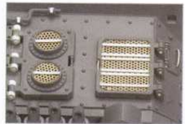
The engine covers have been hinged, and detailed with brass mesh and plasticard strips.
